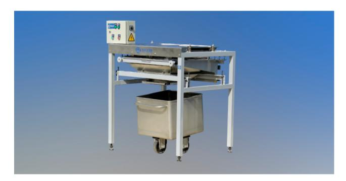
The vibrating sieve is designed for mechanical sieving of dry bulk food products (milk powder, sugar, flour, starch, etc.).
